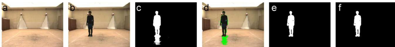
Fig. 3. Foreground extraction procedures. (a) Background image. (b) Current image. (c) Extracted foreground image with shadow. (d) Detected shadow pixels (green color). (e) Foreground image after shadow removal. (f) Foreground image after morphological and filter operations.
